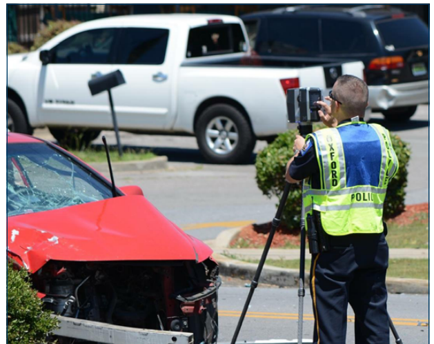
Lt. Don Ridley, Oxford Police Department, scans a crash scene with their FARO 3D X 130 Laser Scanner
