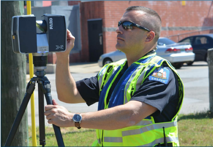
Lt. Ridley, Oxford Police Department, starts up their FARO 3D X 130 Laser Scanner
